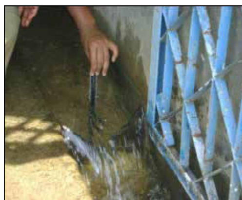
Picture 4 Seepage water flows above V-notch
